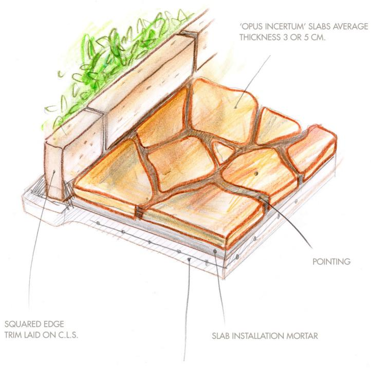
C.L.S. BASE WITH ARC-WELDED MESH 10 CM. THICK
